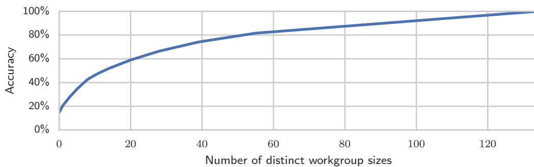
Figure 7.3: Accuracy compared to the oracle as a function of the number of workgroup sizes used. The best accuracy that can be achieved using a single statically chosen workgroup size is 15%. Achieving 50% oracle accuracy requires a minimum of 14 distinct workgroup sizes.
